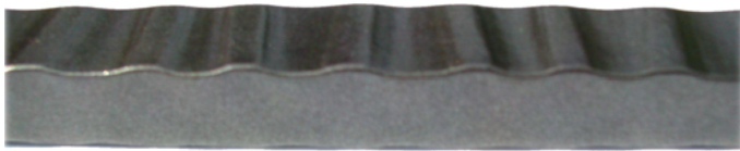
Wavy - with waves on two sides of the bar.
